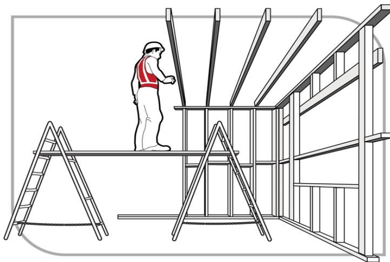
FIGURE 1 INSTALLING CEILING OR UPPER-LEVEL FLOOR JOISTS.
